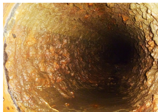
Limescale build-up inside lavatory pipes
