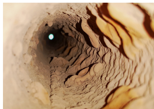
Limescale build-up inside lavatory pipes
